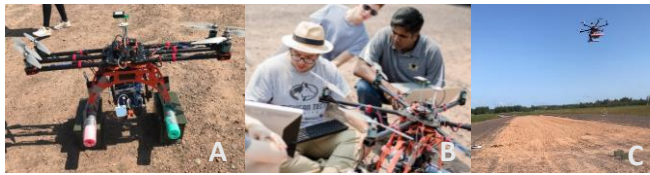
Figure 2: UAV with loaded sensors (hyperspectral and thermal) (A), setup and calibration of the cameras (B), and UAV inflight to record over the Fine Pit (C).
