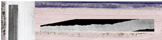
Figure 5: Examples of hyperspectral scans for gradation prediction maps for different soil pits overlaid on DEMs. 2NS pit % sand prediction plot (Left), Coarse pit (Right).
